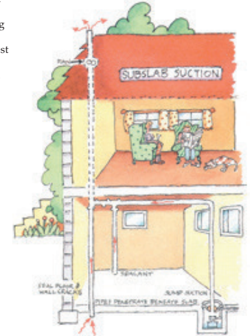
Note: This diagram is a composite view of several mitigation options. The typical mitigation system usually has only one pipe penetration through the basement floor; the pipe may also be installed on the outside of the house.
